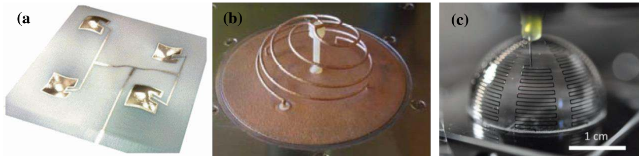
Figure 16: (a) Conformal antenna patterned by sputtering [138], (b) Small spherical wire antenna covered with conductive paint [73], (c) Optical image of an antenna during the printing process [135]
