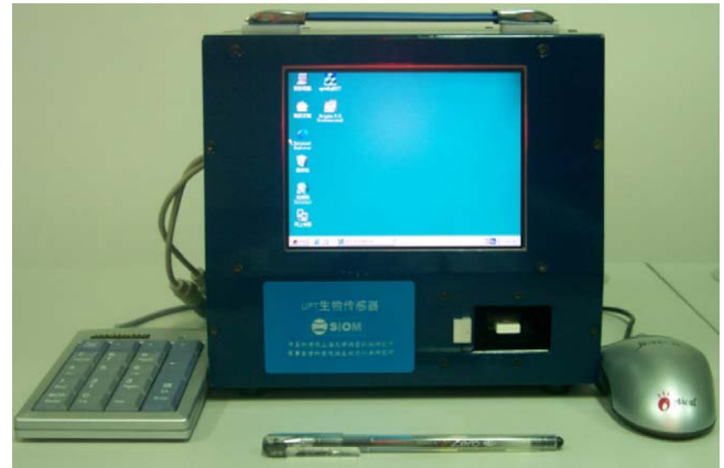
Fig. 2. Photograph of the portable prototype UPT-based biosensor.
