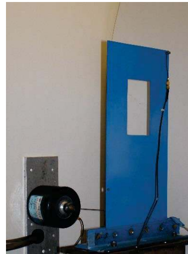
GVT on Article (with a hole for a different test)
