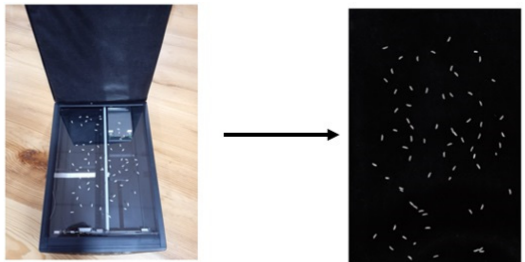
Figure 4. Image of the rice sample acquired from a calibrated flatbed scanner.
