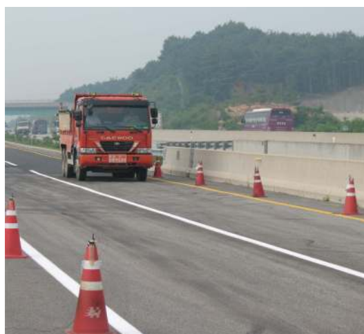
Fig. 7. Vibrations introduced into Yeondae Bridge using a heavy 3-axle truck driving at constant speeds over the bridge
