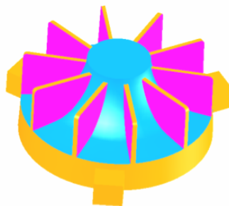
Figure 6. 3D Solid model of an impeller
