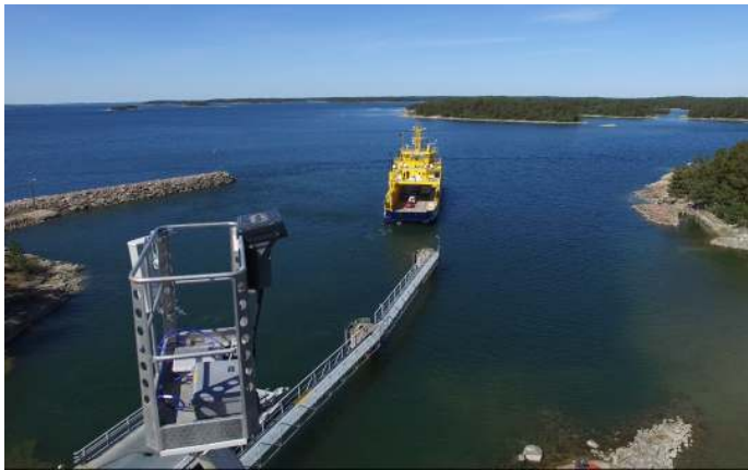
Fig. 3. The 700 MHz transmission antenna installed to a person lift at Kustavi shore.
