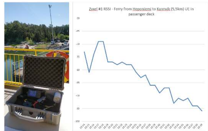
Fig. 9. RSSI measurements conducted on a router on the upper passenger deck, 5 meters above the sea level.
