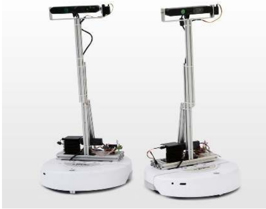
Fig. 12: The two low-cost ( \sim 600\$ ) robots used in our demonstrations: Each robot consists mainly of a differential drive base (iRobot Create), an RGB-D sensor (PrimeSense), an ARM-based single board computer (ODROID-U2), and a dual band USB wireless device.
