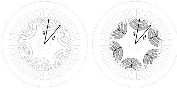
Fig. 8. Structures of a SynRM and a PMA-SynRM.
