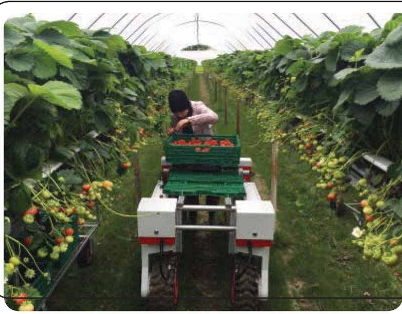
FIGURE 3 The initial trial of a robotic strawberry transportation system in polytunnels (left) and a dedicated design for an on-board picking tray storage (right).
