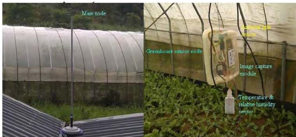
FIGURE 2. WWSN deployed in a greenhouse [3].
