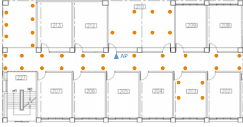
Figure 4—The testbed. Orange dots refer to client locations. Blue triangle refers to the location of the AP.
