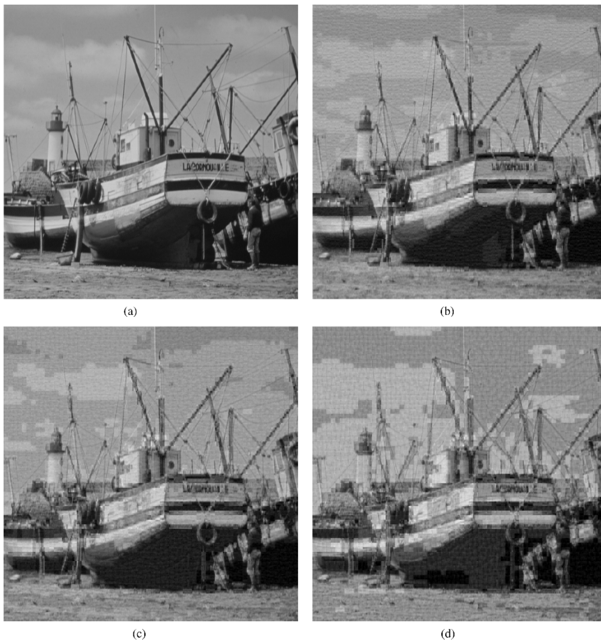
Fig. 14. Rate allocation example. (a) The original Boats image. (b) Original quantized using the 5, 1, 1, 1 rate profile. SSIM index = 0.7743, Laplacian estimate of SSIM index = 0.7865, MSE = 130.28. (c) Original quantized using the 4, 2, 1, 1, rate profile. SSIM index = 0.7551, Laplacian estimate of SSIM index = 0.7676, MSE = 191.62. (d) Original quantized using the 3, 3, 1, 1 rate profile. SSIM index = 0.6689, Laplacian estimate of SSIM index = 0.6704, MSE = 301.39. p = 0.9 . (a) Original. (b) 5111. (c) 4211. (d) 3311.
