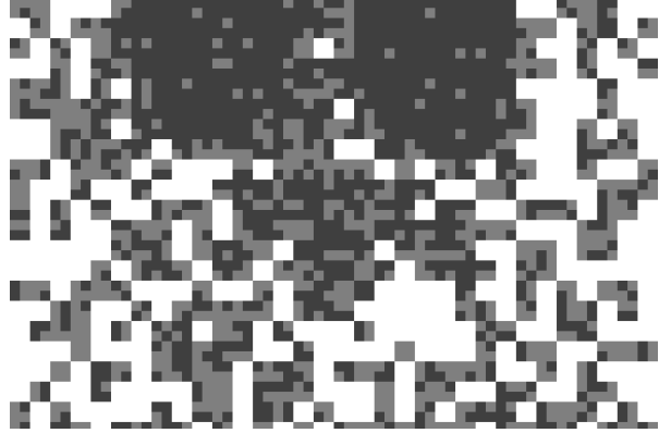
Figure 2. Reconstructed image and coder depth for the image “sergey-zolkin-1045” from the CLIC validation set for \lambda_t/\lambda_e = 0.02/0.0625 . The right image shows the depth of the latent space transmitted at each position, where white indicates the highest depth.
