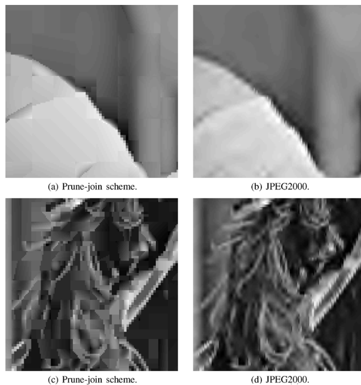
Fig. 17. Comparison of artifacts in two regions of the lena image at 0.15 bpp for the prune-join scheme and JPEG2000.
