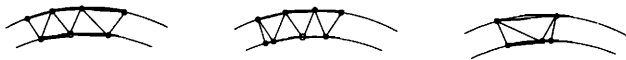
FIG. 2. Illustration of triangulation by angular affinity. Solid circles represent points obtained by the standard homeomorphic mapping. Open circles represent interpolated points.
