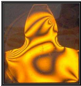
Fig. 19: Test No. 5-(15/28)-pinion-monochromatic light
