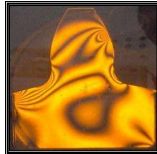
Fig. 15: Test No. 3-(15/22)-pinion-monochromatic light
