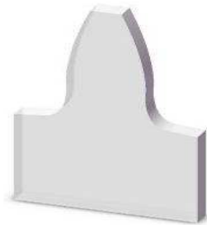
Fig. 7: Specimen of a standard gear with 18 teeth
