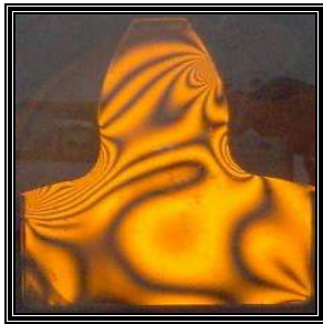
Fig. 11: Test No. 1 (15/18)-pinion-monochromatic light
