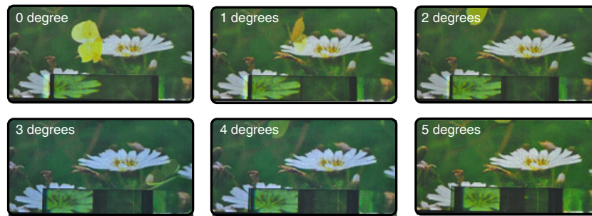
Figure 7 | Characterization of the terrestrial cloak for different observation angles. The observation angle varies from 0^\circ to 5^\circ continuously as the image distortion changes from unnoticeable to noticeable.
