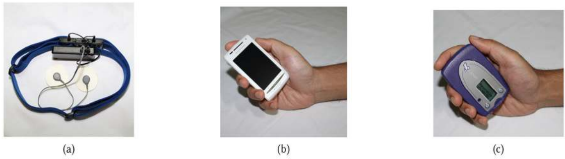
Fig. 2. (a) Chest band sensor. (b) Study phone (Sony Ericsson Xperia X10, Android Smart phone). (c) LENA audio recorder.
