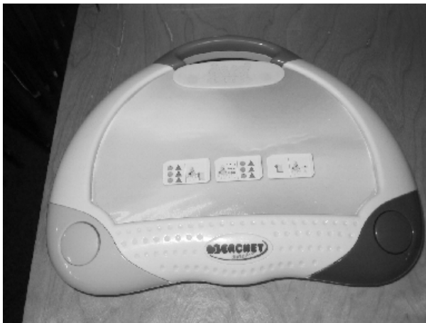
Figure 21: Child-friendly DVD remote-controller from Berchet™, with simple 3-domino overlay sheet to demonstrate potential for implementing Scene-Driver game.
