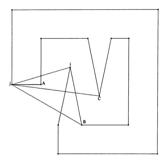
Figure 9: The three possible situations in which path-patching is needed
