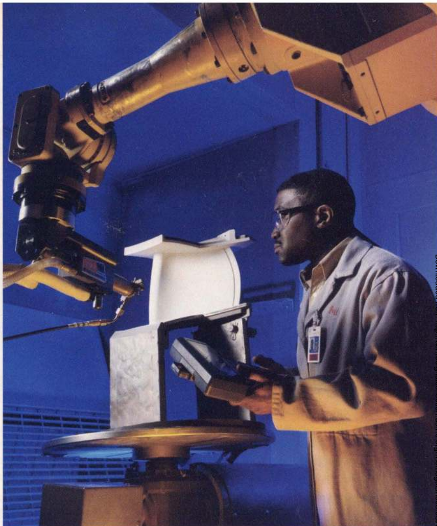
GE's thermal barrier coatings will protect the H gas turbine airfoils when the machine operates at 2,600°F, 200° hotter than its predecessor class firing temperature.
