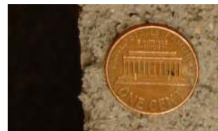
Fig. 17: Image showing the sharp edge and abrasive surface of the cinder block used in the trial described in Sec. VI-D1.
