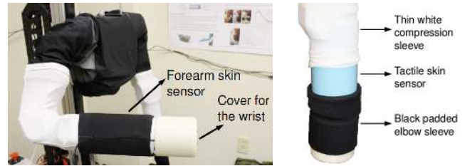
Fig. 9: Left: Tactile skin sensor on the right forearm of Cody (underneath the black neoprene sleeve) as well as a 3D printed cover for the wrist. Right: Two additional layers (thin white compression sleeve and black padded sleeve) that we added on top of the tactile skin sensor (blue) once we mounted it on the robot.
