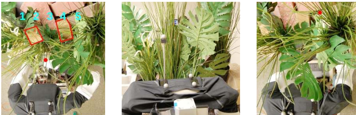
Fig. 18: Left: Five different goal locations that we used to compare the model predictive controller and the baseline controller, described in Sec. VI-D2. The environment consists of compliant leaves and rigid blocks of wood (outlined in red). The red circle denotes the position of the end effector. Middle: View of the foliage from the robot’s perspective. The rigid blocks of wood are occluded by the leaves. Right: Image of the robot after it has successfully reached goal location 5. The red circle denotes the end effector position.
