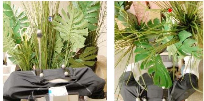
Fig. 1: Left: View of foliage from the robot’s perspective. Two rigid blocks of wood are occluded by the leaves. Right: Image of the robot after it has successfully reached the goal location using the controller we present in this paper. The red circle denotes the position of the end effector.
