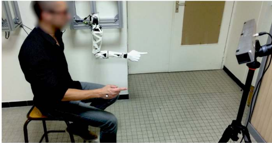
FIGURE 4 | Tele-operation setup, shown during the calibration phase. Subject and robot are placed in the same posture while the Optitrack system (on the left) records the coordinates of the reflecting marker placed on the subject's hand. See this driving mode in operation at https://www.youtube.com/watch?v=Oa9mHMoDtYI .
