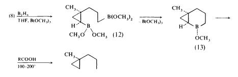
1-Methylcyclopropene and tricrotylborane give predominantly (85–90 per cent) cis-2-(but-3-ene-2-yl)2-methylcyclopropyl-1 di-(2-butenyl)borane (14) along with 2-methylhepta-(2,5-diene-1-yl)-di-(2-butenyl)borane (15) (10–15 per cent). Thus allylborane adds at the double bond in the trimembered cycle via allylic rearrangement while no rearrangement occurs on addition to C<sub>2</sub> and C<sub>3</sub> carbons with cleavage of the ordinary C—C bonding.
