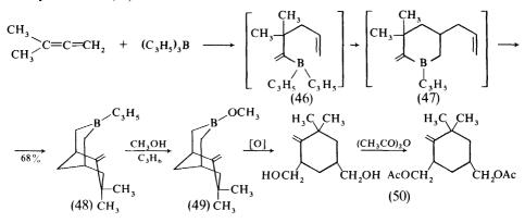
In this case the triallylborane addition to the allenic bond system is similar to that in 1-chloro-3-methylbuta-1,2-diene. However, an intermediate (46) first transforms into boracyclohexane (47) which then undergoes cyclization to the final reaction product (48).
