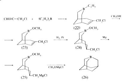
However, in this scheme unexpected complications arose. First of all, it was found that condensation of propargyl chloride and triallylborane yielded (22) with a considerable quantity (4:1) of the isomeric 6-chloro-3-allyl-7-methylene-3-borabicyclo(3,3,1)nonane (27).
