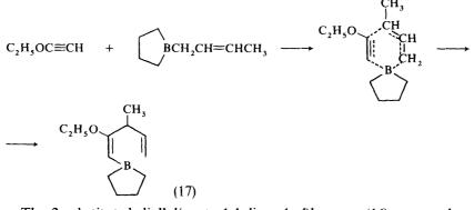
The 2-substituted diallyl(penta-1,4-diene-1-yl)boranes (16) may undergo an intramolecular cyclization to the 3-substituted 1,5-diallyl-1-boracyclohexenes-2 (18). 2-Alkyl-substituted compounds cyclize even at room temperature. The thermally most stable diallyl-(2-alkoxypenta-1,4-diene-1-yl)boranes convert to the compounds (18) only at  $120-130^{\circ}$ .
