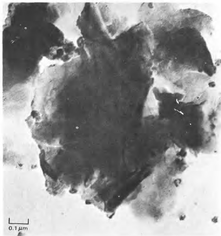
FIGURE 19.—Gibbsite crystallization centers on Wyoming bentonite after 100 days aging.
