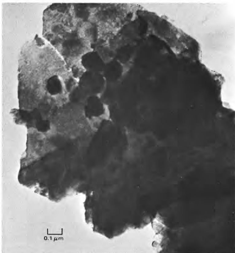
FIGURE 21.—Gibbsite crystals on surface of kaolinite after 100 days aging.
