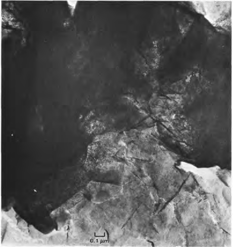
FIGURE 2.—Electron micrograph of Wyoming bentonite.
