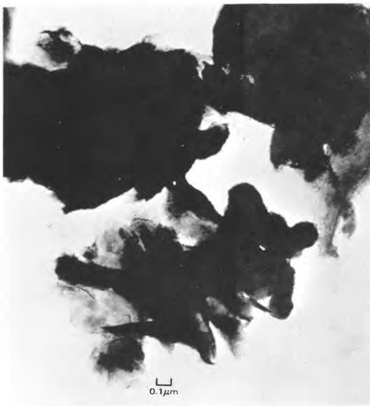
FIGURE 20.—Gibbsite crystals on surface of volcanic ash fragments after 100 days aging.
