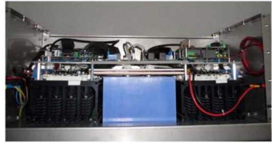
(a). 30 kW prototype converter used to test the PVs local control.
