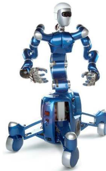
Fig. 1. Mobile humanoid Rollin' Justin of the German Aerospace Center (DLR) with 51 actuated degrees of freedom.
