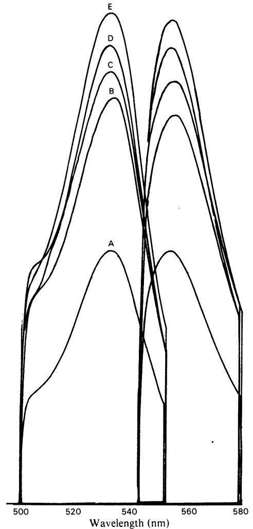
Fig. 1. Fluorescence scans of emission following excitation at 532 nm and of the excitation spectrum giving emission at 553 nm of thiobarbituric acid-reactive material released after iron-dependent free-radical damage to: benzoate (A), deoxyglucose (B), deoxygalactose (C), malondialdehyde standard (6 \mu M) (prepared from hydrolysed 1,1,3,3-tetra-methoxypropane) (D) and deoxyribose (E)
