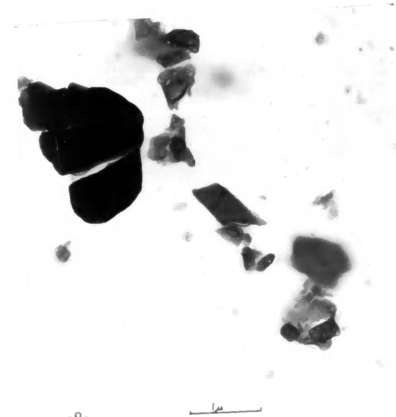
Figure 4.1.9 \text{MgSO}_3 \cdot 6\text{H}_2\text{O} heated on electron microscope hot-stage
