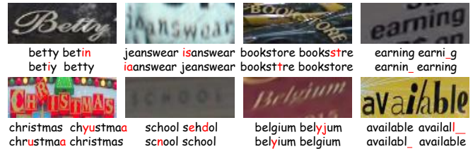
Figure 7. Successful examples using iterative correction. Text strings are ground truth, vision prediction, fusion prediction without iterative correction and with iterative correction respectively from left to right and top to bottom.
