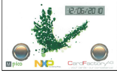
Fig. 1. A Display and Button Equipped RFID Tag
