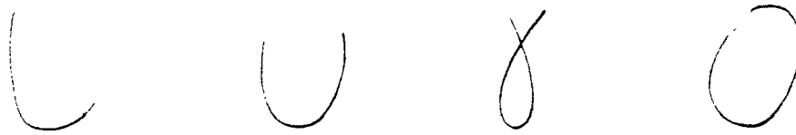
Fig. 4. The four basic stroke types—hook, cup, gamma, and oval. All cursive characters can be represented as combinations of strokes belonging to this set, with the addition of a straight-line stroke.
