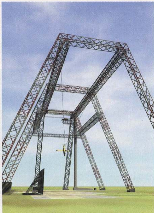
A 3-D computer simulation of an impact dynamics facility can test airplanes and other flight craft for crash safety, including how design changes can protect passengers and increase their chances of survival.
