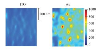
FIG. 2. (Color online) Local field intensity  $\mathbf{E}^2(\mathbf{r})$  at rough (random Gaussian roughness, MRS 50 nm) surfaces of ITO ( $\varepsilon = 0. + i0.57$ ) and gold (dielectric data are adapted from Ref. 31). The excitation radiation is p-polarized incident at 45°. The color scale of intensity (relative units) is indicated to the right of the panels.
