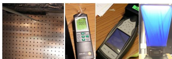
Figure 4. Equipment used, from left to right: a mounted hose and the manometer, sound meter, balometer
