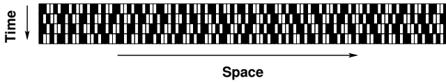
Figure 3: A four-frame sequence of projected patterns. Each pattern has 110 stripe boundaries (111 stripes), with the property that each stripe boundary has a unique code (consisting of the black/white illumination history on either side of the boundary over the sequence of four frames).
