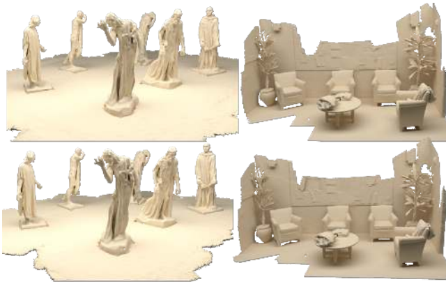
Figure 10: Comparison of output meshes from our online method (top) with the offline method of [Zhou and Koltun 2013] (bottom).
