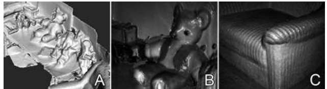
Figure 10. A: the PMD scene acquired with a PMD ToF camera. B and C: close-ups using per-pixel intensity values for coloring.
