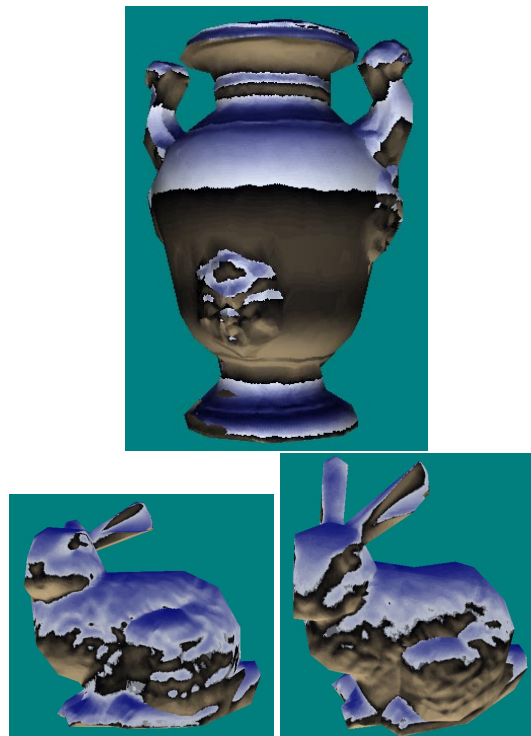
Figure 7: Examples of bump-mapped objects rendered using a chrome effects. In this example the color is assigned by taking into account the reflection of a typical landscape (brown below, and blue above).
