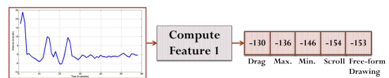
Figure 5: Extraction of the sketch-gaze distance feature in the dynamic system. For a given signal, its log probability of being generated by each of the HMMs is calculated and the degree of likelihood is used as an informative feature for classifying activities.
