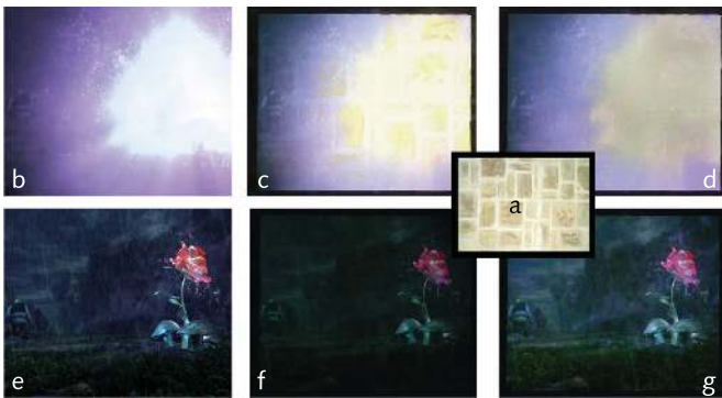
Fig. 9. Two frames of an animation (b, e) projected onto a natural stone wall with a static radiometric compensation (c, f) and with our adaptive algorithm (d, g).
