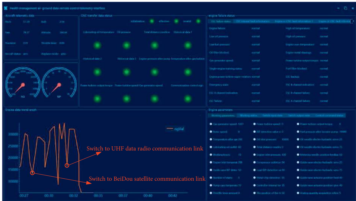
FIGURE 17: Display of the UAV/engine data switching between three communication links.
