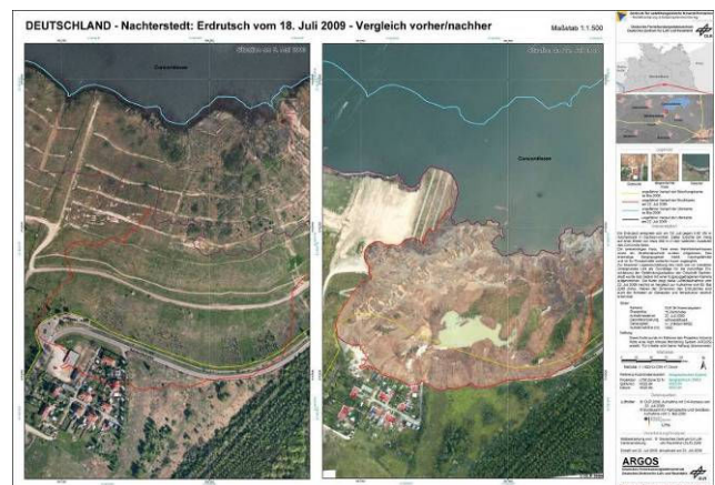
Figure 3: Map of the situation at Nachterstedt prior to (left) and after the landslide (right). It was produced at DLR Center for Satellite Based Crisis Information (ZKI). Right part shows a mosaic of 3K camera aerial images. Red line shows the landslide border, blue line marks the original and purple line the new waterside border. Yellow line is the approximate border of the slope.
