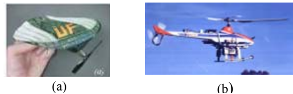
Figure 1. (a) University of Florida fixed wing micro air vehicle, (b) YamahaR50-based autonomous helicopter
