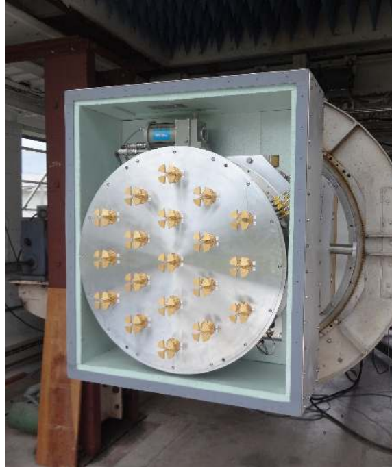
Figure 3.2: The L-band PAF receiver in the outdoor test facility at GBO. This instrument is placed at the feed of the Green Bank Telescope.
