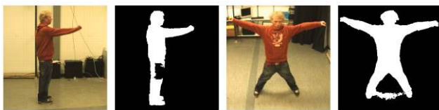
Fig. 1 Examples of silhouettes which are used for classification. Note the holes in the segmentation and the artifacts due to reflections on the floor
