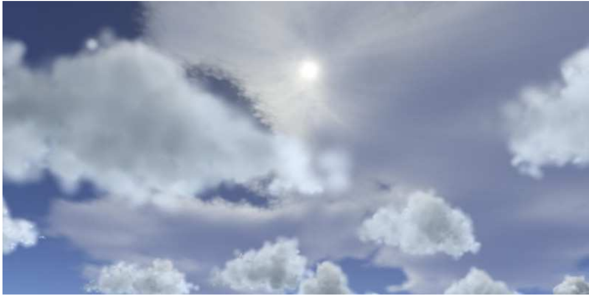
Figure 6.4: These static particle-based clouds were rendered with isotropic scattering, and therefore lack the bright edges visible in real clouds.
