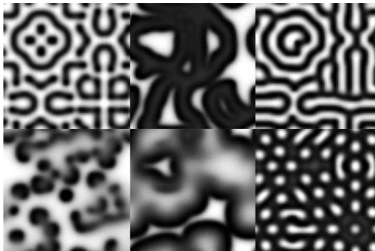
Figure 4.16: The result of the 2D gray-scott reaction diffusion with varying parameters. By varying the fixed-point computation precision we determined that 14 bits of precision were sufficient to approximate the results of a 32-bit floating point simulation. With the advent of floating point GPUs, this is no longer necessary (see Section 4.3.7).
