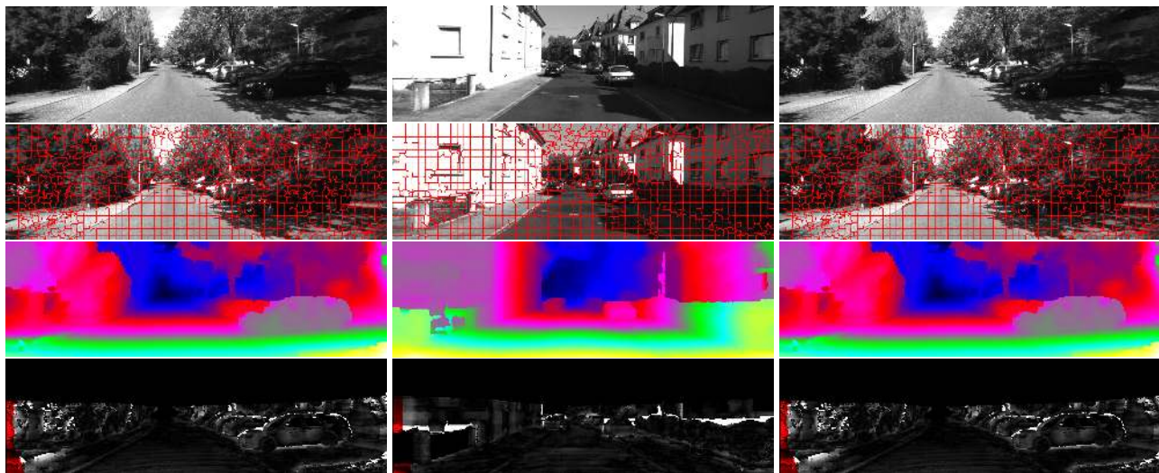
Figure 11. KITTI: Our results on the KITTI dataset. Top row shows the image, second row the super pixels, third row the disparity estimates while the errors are displayed in the last row.
