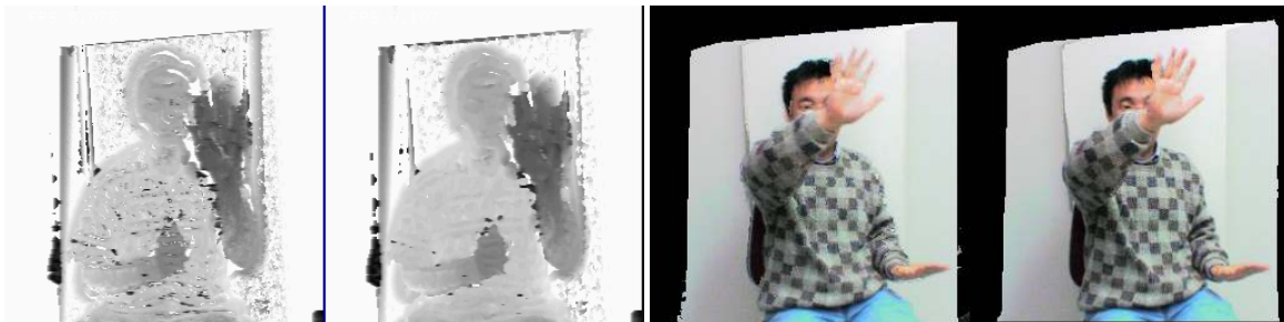
Figure 9. Impact of support size on the depth and color reconstruction; For each pair, the one on the left uses a 1 \times 1 support window (real-time results) while the one on the right uses a 5 \times 5 support window.
